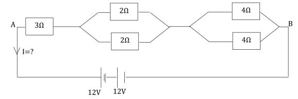
In the above circuit, calculate the current flowing through the circuit
